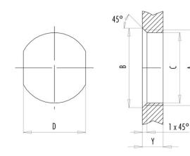
Installation direction: o-ring sits on chamfer.
